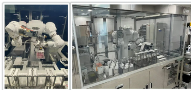
All Figures are courtesy of the author. Figure 1. The Maholo robot automates cell culturing and differentiation.
